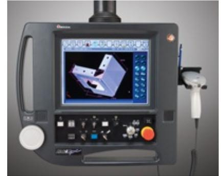
Standing at a new machine controller, the operator touched the screen to open the program, showing a tool setup sheet with all information regarding tool type and part layout. The control then graphically guided the operator through the setup process. Programs were downloaded directly to these new machines, effectively eliminating all time previously spent entering data (see **Figure 3**).
